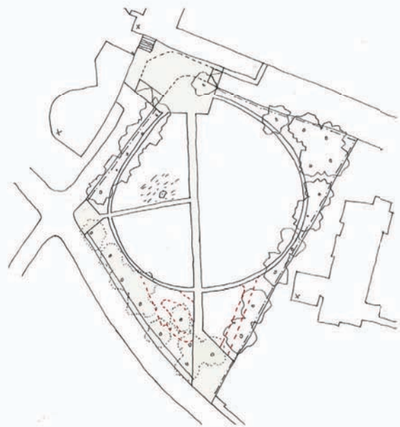
Fig. 6.55: Sketch of Lowlands recreation ground showing improved connectivity with Harrow-on-the-Hill Station, improved entrances, new diagonal paths and raised tree canopies to improve accessibility
